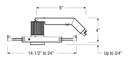
Field Cuttable Ceiling Cut-out: 2-3/8" Ø
