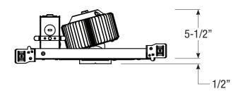
Field Cuttable Ceiling Cut-out: 2-3/8" Ø
