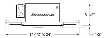
Field Cuttable Ceiling Cut-out: 2-3/8" Ø
