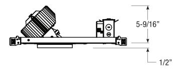
Field Cuttable Ceiling Cut-out: 5-1/8" Ø
